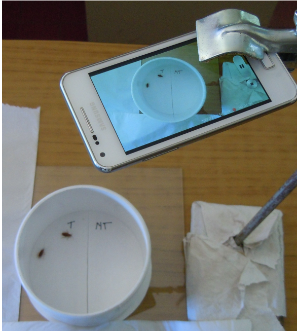
Figure 1: The mobile version of the system, capturing video before processing it. This is all the setup required by the zoologists to test the EOs repellent effect.
